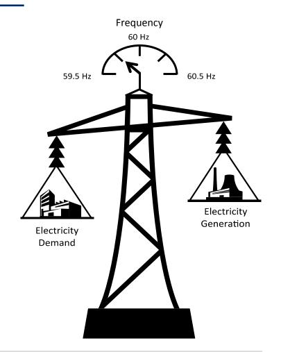
Maintaining system frequency is one of the fundamental drivers of power system reliability
