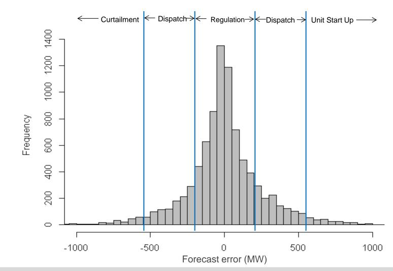
The system was designed to accommodate small amounts of uncertainty. Large forecast errors are the most costly.
