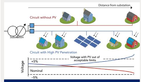
**Figure 1:** An illustration of the increased voltage range in systems with high PV penetration. On a circuit with no PV present (red line), the voltage along the feeder decreases as distance from the substation increases. If the PV power injected into the circuit (blue line) is high enough, the voltage will increase, potentially raising the voltage above normal operational conditions.
