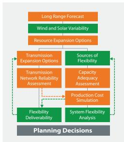
Key steps required for traditional power system planning are indicated by the orange boxes above [1]. Integrating variable renewable generation requires an evolution to the planning process to include the new analyses and approaches, indicated by green boxes. This new planning framework can facilitate higher levels of variable renewable energy (VRE) integration while maintaining system reliability and cost-effectiveness.
