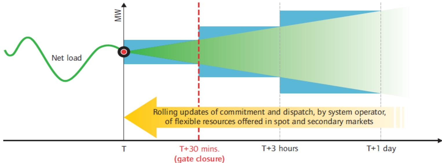
T: Time of operation (instant when electricity is produced and consumed)
