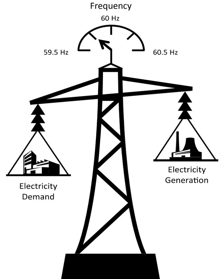
***Maintaining system frequency is one of the fundamental drivers of power system reliability***
